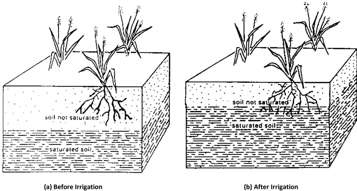
**Figure 1. Groundwater table before and after irrigation**
