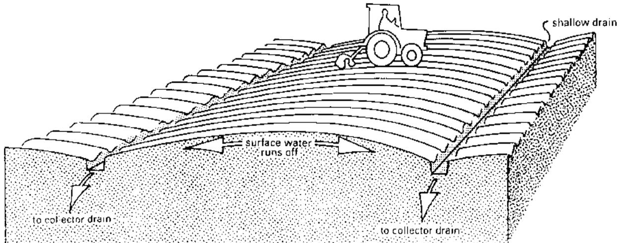
**Figure 2. Surface drainage- The field is given artificial slope to facilitate drainage**
