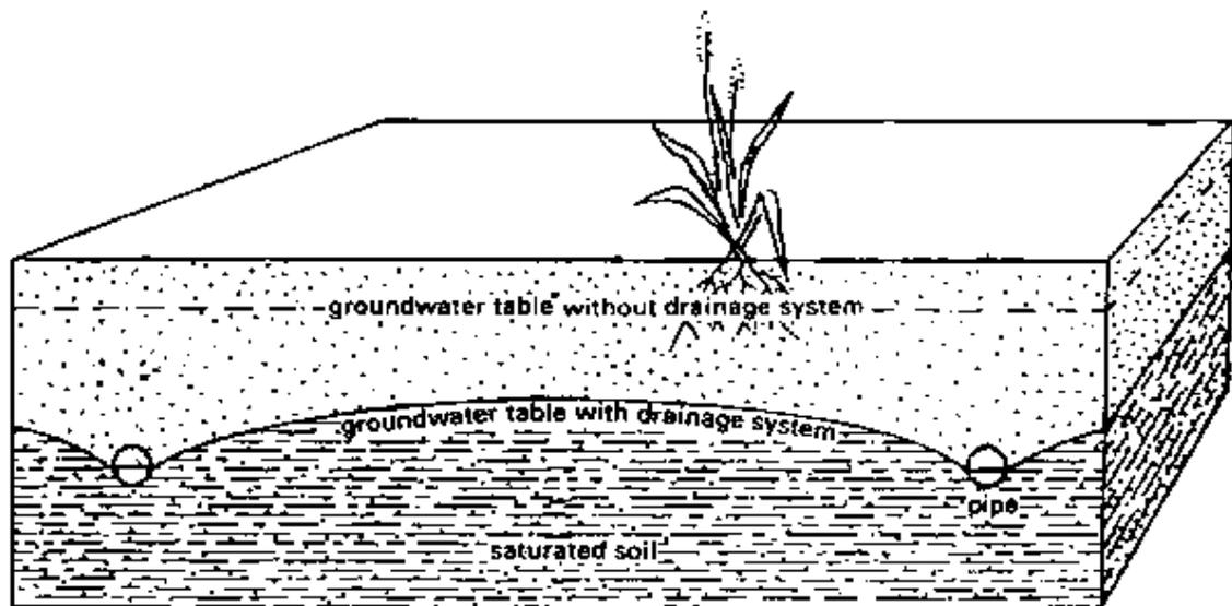
Figure 4. Pipe drains
